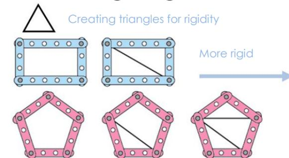
Making small-scale frame structures
